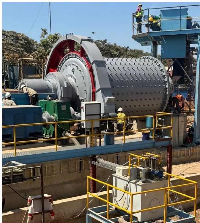
Figure 3c: Buckreef Gold's 1,000 tpd Ball Mill
