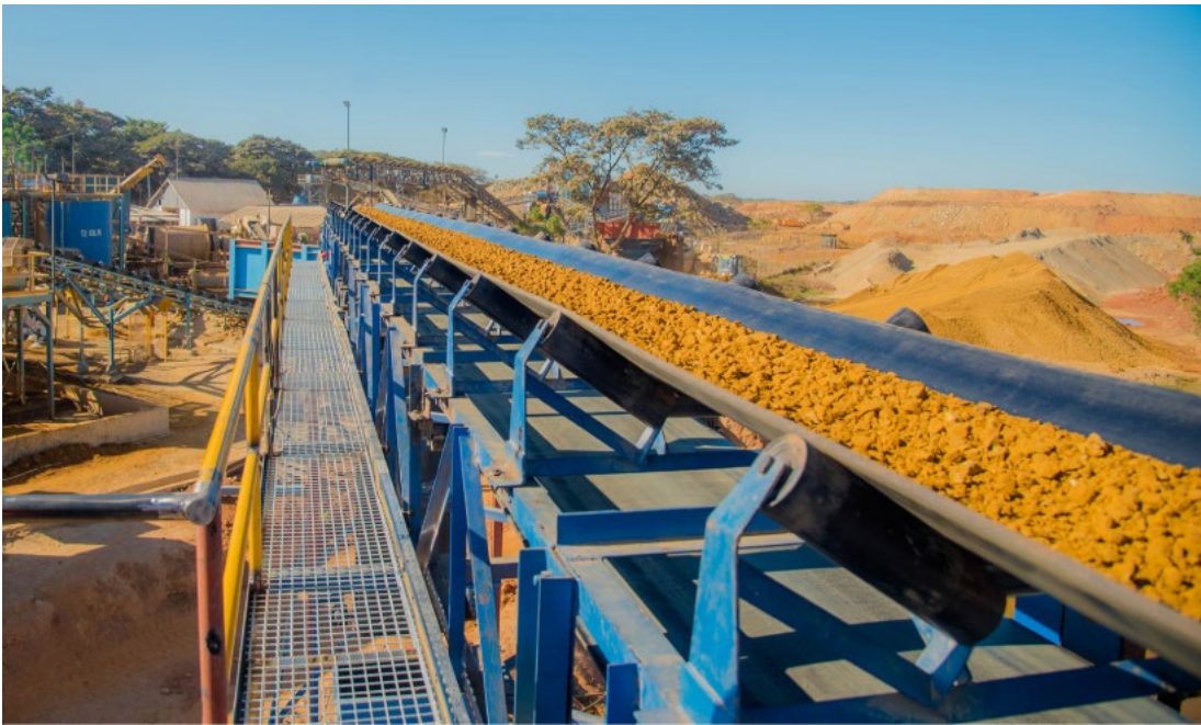
Figure 3: Buckreef Gold Ore Moving Through Crushing Circuit
