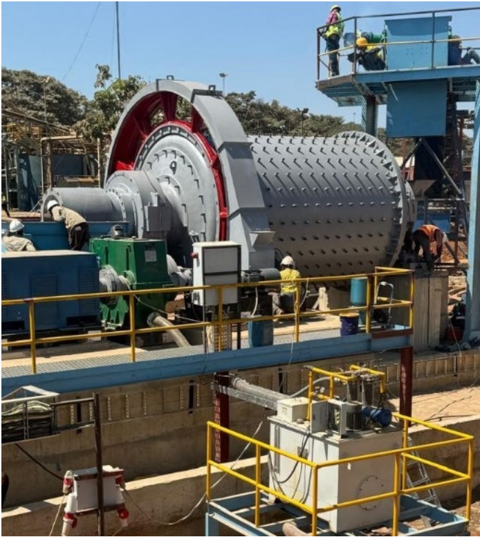
Figure 4: Buckreef Gold's 1,000 tpd ball mill
