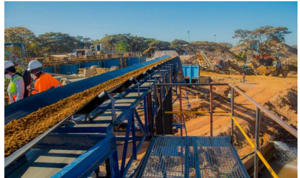
Conveyor transporting ore at Buckreef Gold Mine
