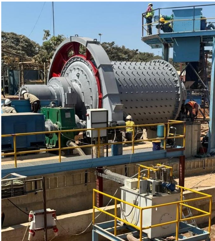
Figure 3c: Buckreef Gold's 1,000 tpd ball mill
