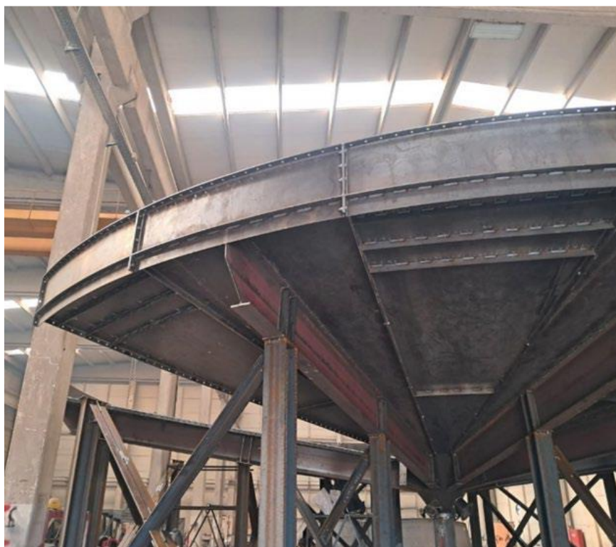
Figure 5: 18 Meter Diameter Pre-Leach Thickener
