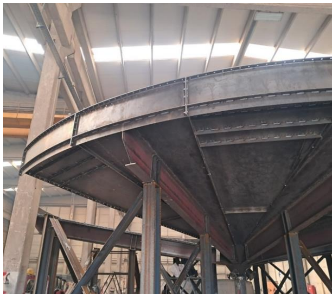
Figure 8: 18 Meter Diameter Pre-Leach Thickener
