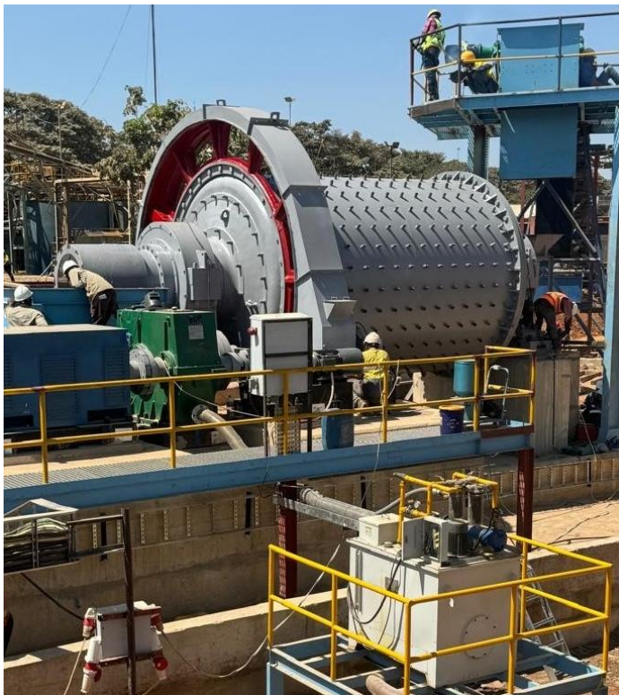
Figure 3c: Buckreef Gold's 1,000 tpd ball mill (Q3 2024)
