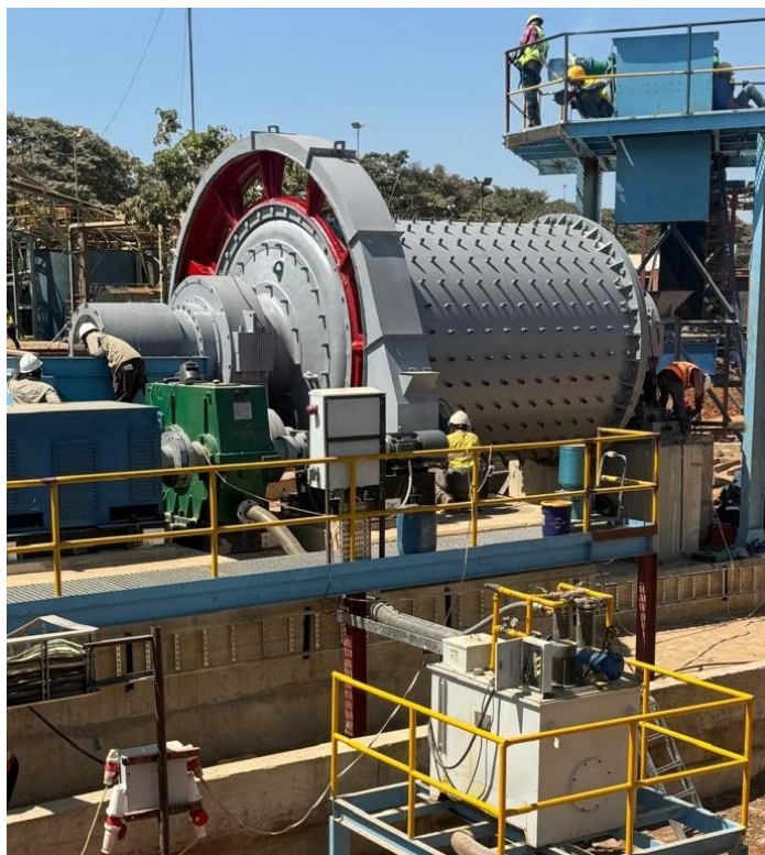
Figure 3c: Buckreef Gold's 1,000 tpd ball mill (Q3 2024)
