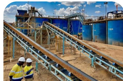
2,000 tpd Processing Plant at Buckreef Gold, showing CIL tanks and conveyor feed to the ball mills
